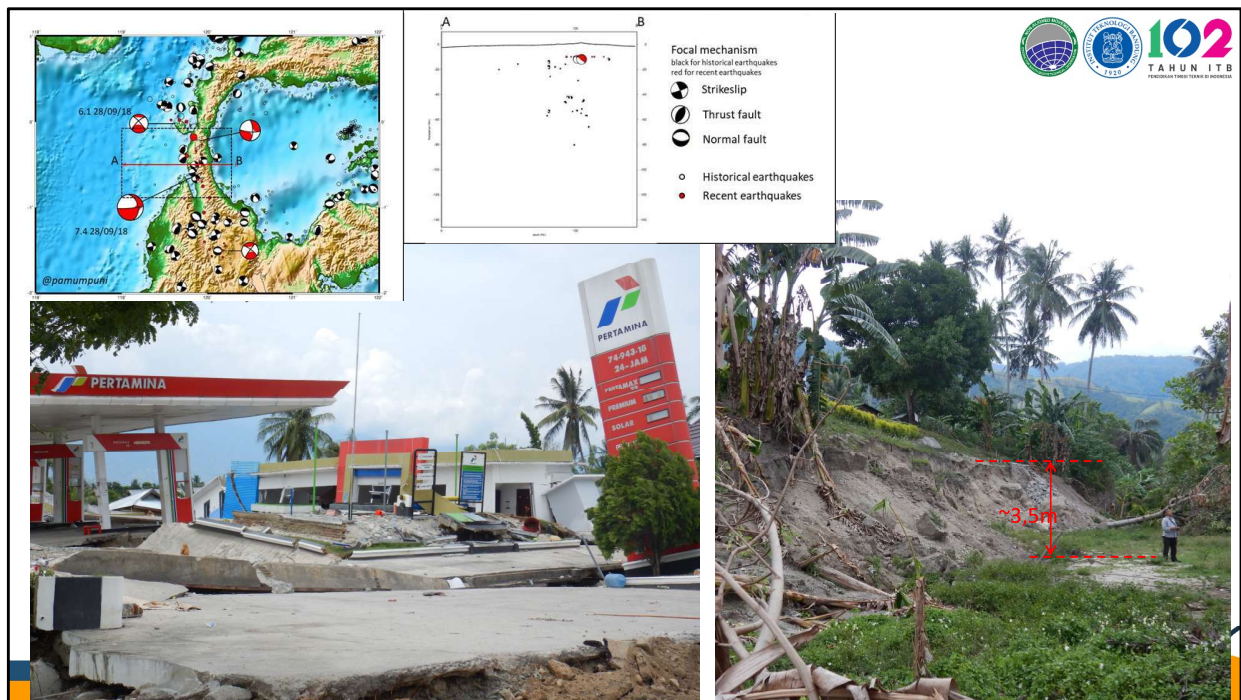
Example of liquefaction following Palu earthquake in 2018 (left) Surface rupture showing vertical displacement more than 3.5m (right)
